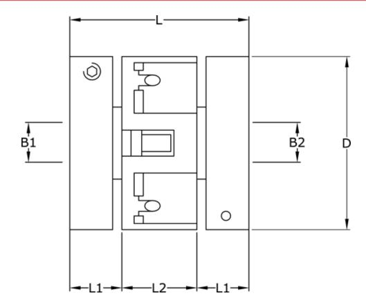
$\begin{array}{lll} B1 & = 6 \\ B2 & = 6 \\ D & = 27 \\ L & = 25.4 \\ L1 & = 9.3 \\ L2 & = 6.9 \\ Screw = M3 \end{array}$
